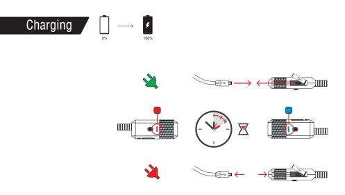
Before using your Shad HANDSFREE device for the first time, you must charge the device completely. Connect the terminal (1c) to the provided USB charging cable (4) and then connect the cable to a USB charging port. While charging, the red LED light will switch on (1a) and it will change to blue once charging has been completed.
