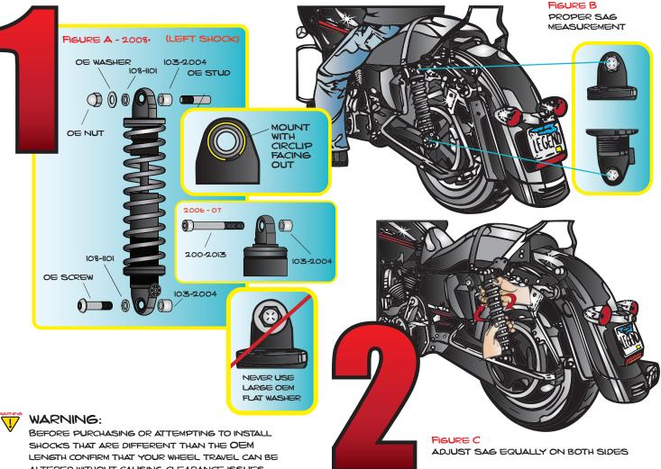
ALTERED WITHOUT CAUSING CLEARANCE ISSUES SUCH AS, SWING ARM / AXLE TO EXHAUST CONTACT AS WELL AS CHAIN/BELT GUARD OR TIRE CONTACT.
