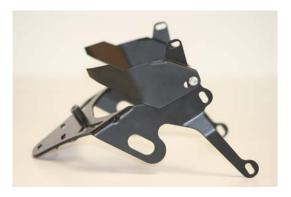
Before refitting seats fit triangular spacer panels, using M5 OEM bolt through 6mm (rearmost) slot in panel spacer and front M5 tapped hole in exhaust cover (plastic) and M6 button head screw and lock nut through front slot of panel spacer and 6mm rearmost hole in R&G tail-tidy. These are fully adjustable and should be adjusted to hide exhaust heat shield and follow the appearance of the bike.
