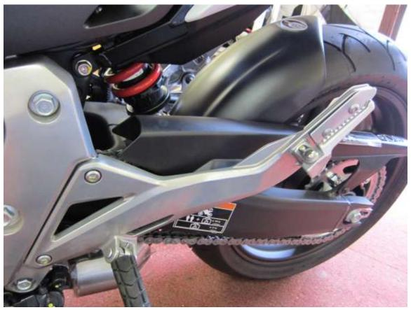
• Finally replace the Honda footrest and retighten retaining bolts to original torque settings.
