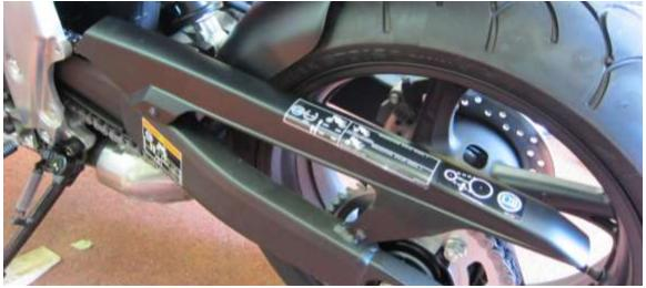
• Replace the original chain guard back onto its mounts, the front of which will overlap the hugger final fixing mount. Using the original bolts reattached the chain guard.
