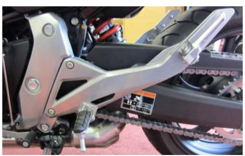
• Unscrew Left Hand Side Footrest Bolts using an 8mm ALLEN key or ALLEN socket.
