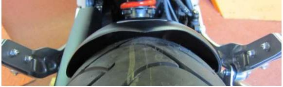
• Finally check hugger for proper fit and spacing, ensuring the hugger is not touching the rear wheel. Double check all fittings and retighten where needed.
