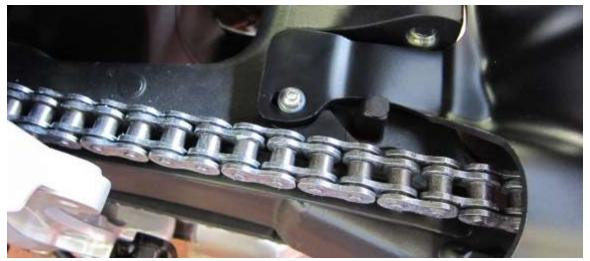
Using the remaining bolt and washer supplied in the kit (M6x25mm button head bolt and M6 washer) screw in the top locating bolt.
