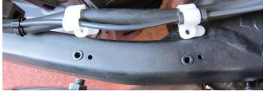
• On the right hand side of the swingarm, using a screwdriver remove the two M5 crosshead bolts from the swingarm and cable retainers.
