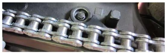
• Using a 8mm socket remove the M6 bolt holding the swingarm guard in place.
