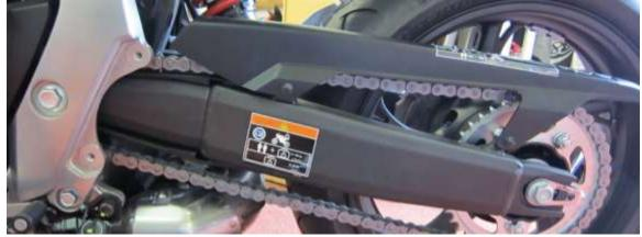
• Using a 8mm socket or spanner unscrew the two hex head bolts holding the chain guard in place and remove it. **Keep the screws these will be needed upon reassembly.**
