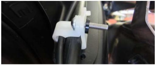
Using the two M5 x 25mm bolts, washers and the S0455 spacers (supplied in the kit) place them through the cable retainers with the spacer going on the underside of the cable retainer. Line up those bolts through the holes in the hugger with those in the swingarm and tighten both bolts down.
