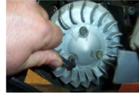
RETIRER LES 3 VIS SUPPORT DE VENTILLETTE AVEC UNE CLÉ ALLEN DE 5 ET LA DÉPOSER.
