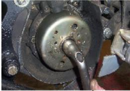
DESSERRER L'ÉCROU DU ROTOR AVEC UNE CLÉ A PIPE.
