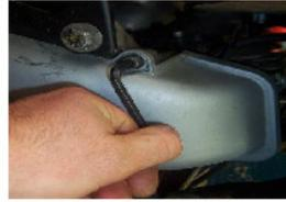
POUR LES MODELES A REFROIDISSEMENT A AIR, RETIRER LES VIS SUPPORT DU CACHE ALLUMAGE AVEC UNE CLÉ ALLEN DE 5 ET LE RETIRER.
