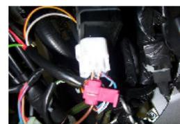
PRÉSENTER LE CLIP ROUGE FOURNI SUR LE CABLE MARRON DU CDI D'ORIGINE ET PLACER LE CABLE MARRON DU DIAGRAMME DANS LE DEUXIÈME EMPLACEMENT DU CLIP ET LE FERMER AVEC UNE PINCE POUR METTRE EN CONTACT LES 2 CABLES MARRONS.
