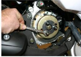
TOURNER LE ROTOR A LA MAIN POUR VENIR METTRE LE PISTON EN CONTACT AVEC SON BLOCAGE, DÉMONTER LES 3 ERGOTS DE POMPE A EAU AVEC UNE CLÉ PLATE DE 10.
