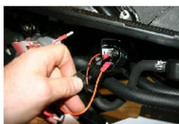
DÉVISSER AVEC UNE CLÉ A PIPE DE 10 LA VIS SUPPORT DE LA BOBINE HAUTE TENSION D'ORIGINE ET PLACER LE CABLE NOIR COSSE RONDE A LA MASSE DE LA BOBINE ET RESSERRER AVEC LA VIS DÉMONTÉE ET BRANCHER LE CABLE ORANGE DU DIAGRAMME SUR LA BOBINE HAUTE TENSION.
