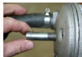
ENLEVER LE BLOQUE PISTON ET REPOSITIONNER LA BOUCIE A SA PLACE AVEC SON ANTI PARASITE.
