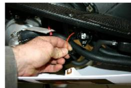
RETIRER LE CABLE ORANGE DE LA BOBINE HAUTE TENSION D'ORIGINE.
