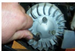
POUR LES MODELES A REFROIDISSEMENT A AIR, REPOSITIONNER LES 3 VIS D'ORIGINE SUPPORT DE VENTILLETTE AVEC UNE CLÉ ALLEN DE 5.
