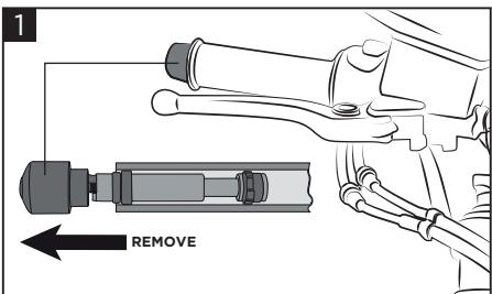
**Remove the originals counterweight and internal weight.**
