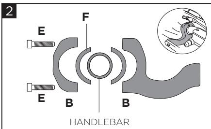
**Mount the bracket (B) on the handlebar using screws (E) and use the spacers (F).**
