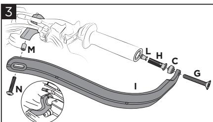
**Fix the bar (I) to the handlebar using the expander (H), the insert (L), the spacer (C) and the screw (G) as shown in the figure. Fix the bar to the bracket using the bushing (M) and the screw (N).**
