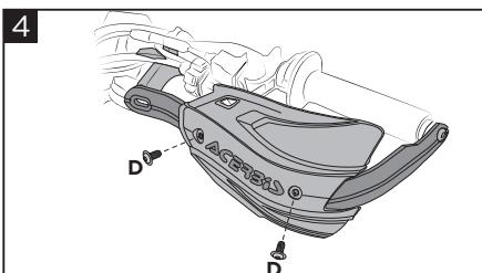
**Assemble the cover to the bar using the screws (D).**
