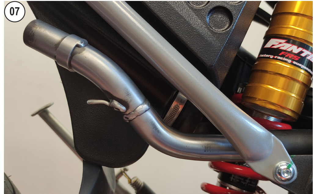
07 INSTALL THE PIPE
