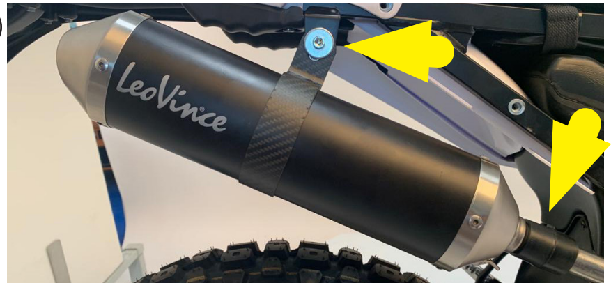
INSTALL THE LV MUFFLER - REMEMBER THE RUBBER SLEEVE
