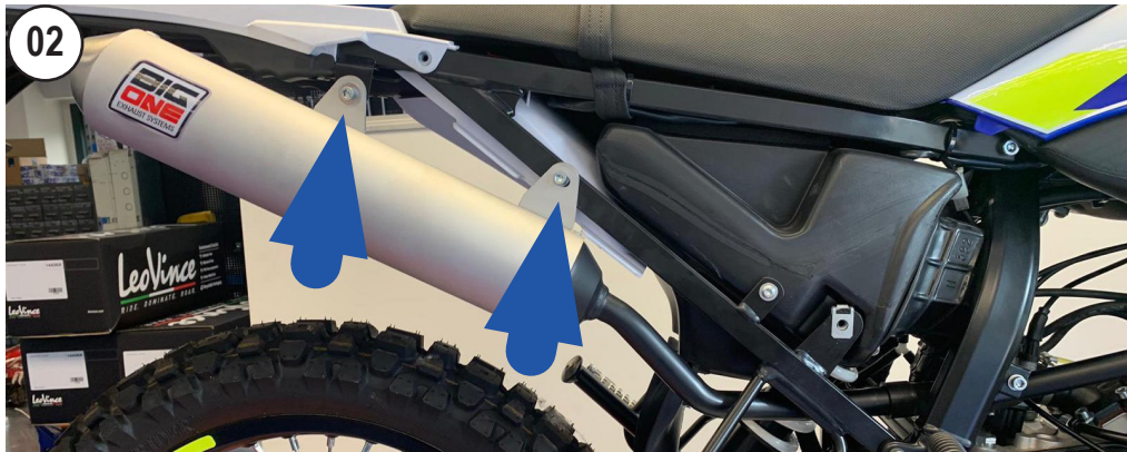
UNSCREW AND REMOVE THE ORIGINAL MUFFLER
