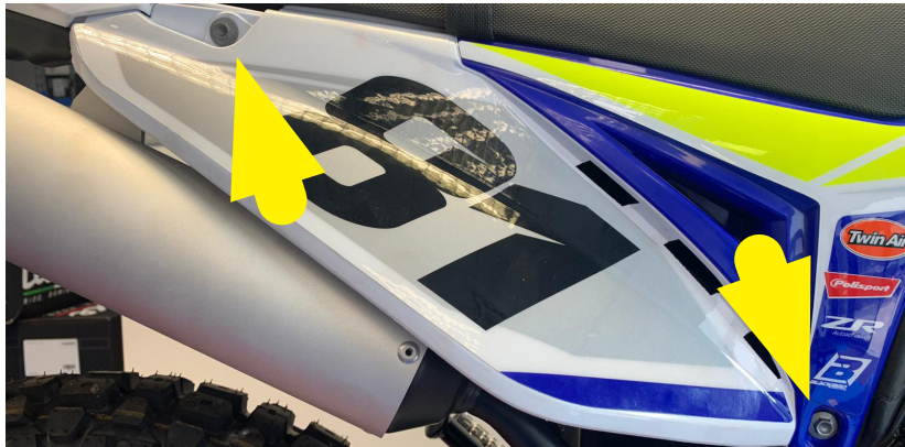
UNSCREW AND REMOVE THE SIDE PANEL
