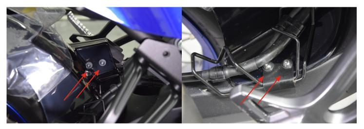
Remove the bottom of the protective film and place the hugger.
