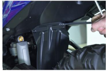
Remove the protective mudguard on the rear wheel as shown in the photo. You will not use the screws and the mudguard again, so you can save them if you want to restore it at the original form
