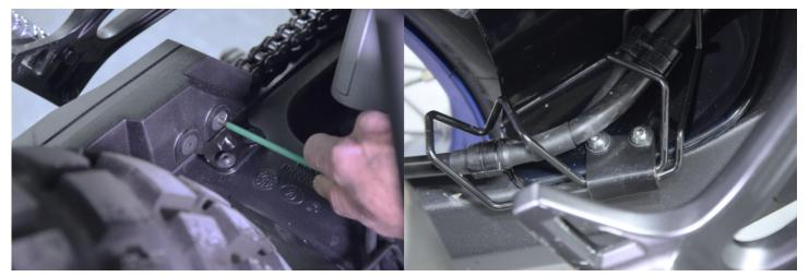
Then remove the screws that secure the chain guard to the inside only. You will not use these screws again (left photo).
