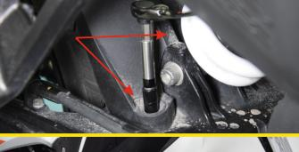
Then remove the two main screws. (In the third photograph there is only the right side, on the left side there is the same screw)
