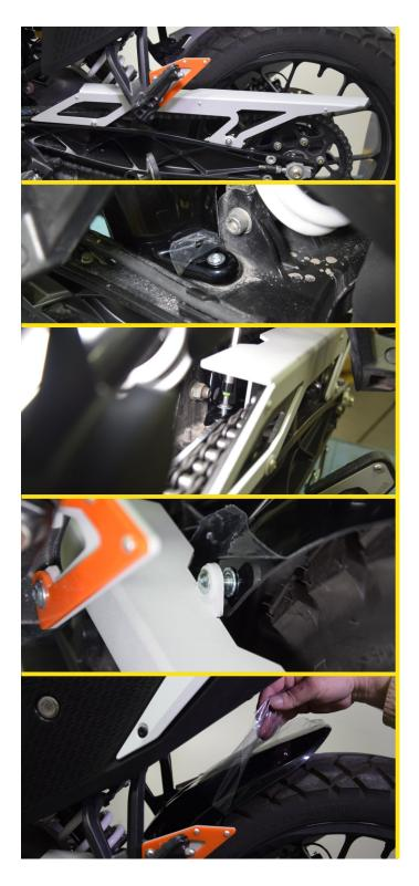
Put the chain guard in place and pass the screws (blueprint 7-10 forward & 5-8-9-11 for back) without tightening them, just touch them to hold the product in place.
