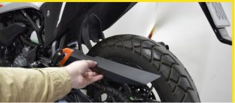
After you have removed all the screws you must open the back side of the chain guard which covers the base on which it was mounted, to get it through from the chain. Then rotate the fender and because it is elastic you can carefully/easily remove it.
