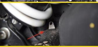
After that remove the nut, (not easily seen). (In the second photograph you will see the place of the nut, only seen from the right side under the shock ubsorber.)
