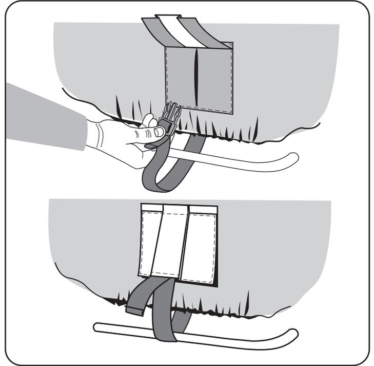
In case of inclement weather use the included rain cover to protect your bag. After the bag is completely covered and the bottom bungee wraps around under the bag, secure the rain cover using the side attachment straps. Pass the strap with the male buckle around the luggage rack or frame, lift the rain cover flap and insert the buckle through the slot and reconnect into female buckle under the cover. Fasten the cover flap closed. Repeat on all 4 straps on the bag.
