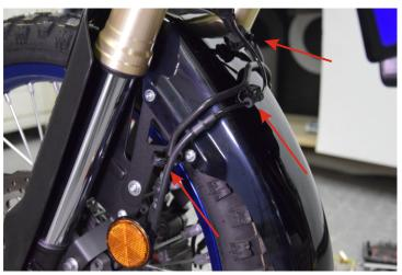
Carefully insert the fender at the position of the old one. Be careful with the tubes it will be difficult to pass those again in the correct position inside the clips.
