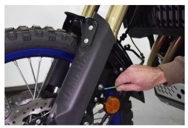
Then tighten the remaining screws that secure the fender. Before tightening, make sure that the part is properly aligned. When you have tightened all the screws, place the hoses in their exact position and close them by pressing each one separately.
