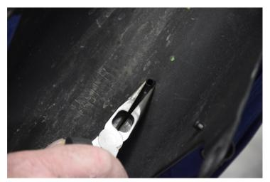
When you remove it, turn it upside down and with a small pair of pliers, (as demostrated in the photo) lightly press the clips from the inside to remove them from the fender. Be sure to keep those for the new mud guard.
