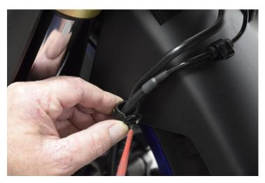
Before removing it from the motorcycle, open the clips that hold the front brake hose and the ABS cable with a small straight screwdriver. Carefully open them and remove the above, pipes and cable. Carefully pull the fender forward to escape from the tubes and pass between the forks.
