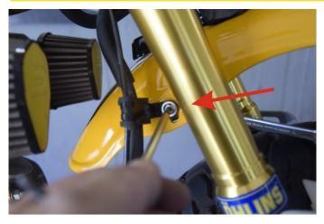
Finally fit the other screw with the washer and the nut in the middle to hold them and tighten it.
