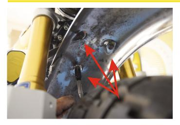
Remove the 3 screws holding the fender at the bottom and remove it from the motorcycle.
