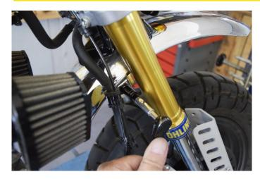
Remove the screw that holds the tubes of the front brake.
