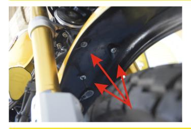
Place the new fender in place of the old one and screw it with the new screws that are in the package and tighten it well.
