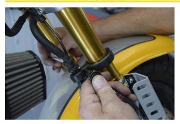
Finally screw the base for the brake pipes. Place it directly under the old stand as shown the photograph.
