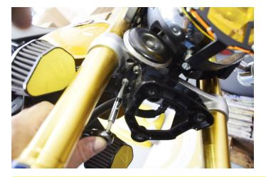
Remove the base the fender was screwed. It has 4 Allen screws on the 4 corners of the base.
