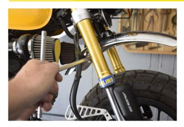
Unscrew the screw that holds the tubes for the front brake and ABS.
