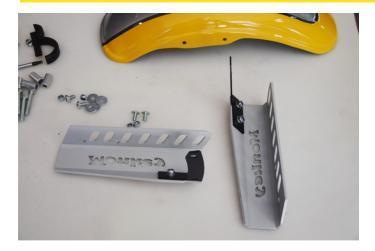
Now you have to prepare the fender before mounting it. First place the 2 supporting brackets on the fork guards, as shown in the photo.
