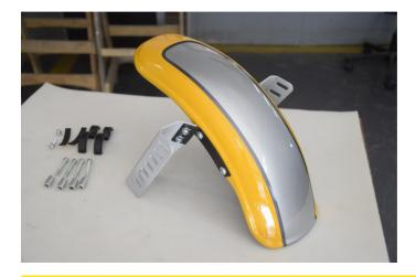
Then place it on the fender. Use the screws provided in the package. Align it and tighten it well.
