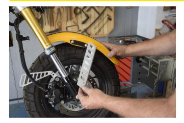
Place the fender between the front suspensions, as the photo shows.
