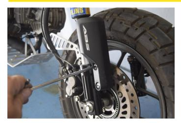
Remove the two screws holding the guard in place of the front suspension. Do the same on the other side side.
