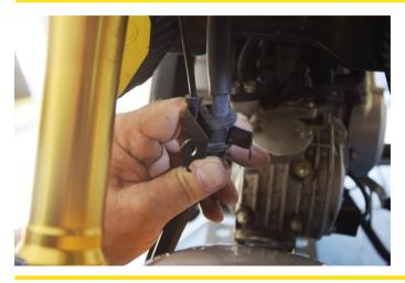
Remove the supporting brackets from the front tube brake. To do so you need to open it as shown at the photograph.
