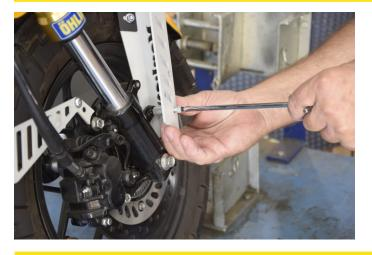
Pass the adapter between the bottle and the reed guard and tighten the screw without tightening it.
