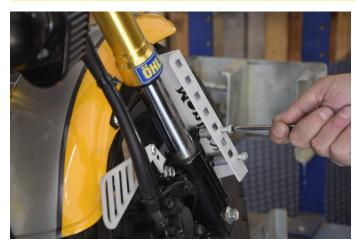
Do the same forthe top screw. Continue with the other side and after you put all the screws, check if it is aligned, then tighten all screws.
