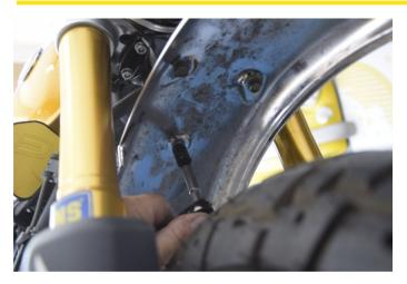
Unscrew the 3 screws holding the front fender from the bottom of the fender and remove it from the  $\,$ motorcycle.
