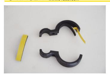
To complete the preparation, stick the adhesive foam on the new base to prevent any damage on the front suspespions.
