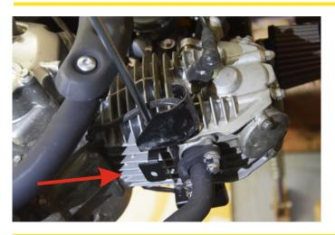
Remove the sensor protector from the right side and insert the relevant bracket from the inside, as shown at the photo. Screw it but do not tighten it yet.
