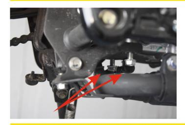
Remove the two screws on the back of the engine.
