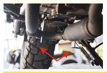
With the same screws, install the two supporting brackets as demostrated. Make sure they are parallel and tighten them.
