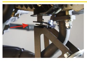
Pass the last bracket between the upper ones you have put on the engine and underneath which are placed on the rack. Here you will use the large screws (M6X15). Now you can tighten them normally.
