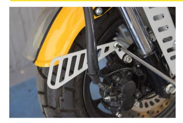
Place the new guard in the same position as the old one. Screw it in with the new screw provided in the package and tighten it well.
