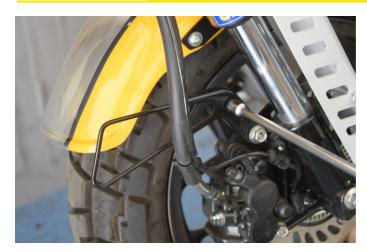
Remove the screw holding the old protector and remove the it from the motorcycle.
