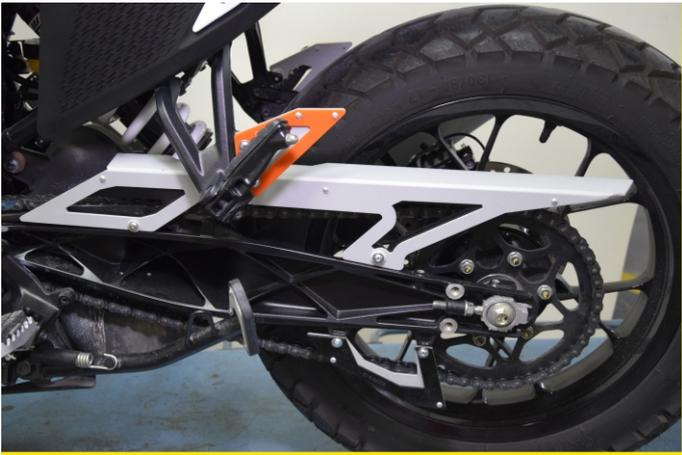
Put the chain guard in place and pass the screws (profile 4-8 front & 3-5-6-7 for back) without tightening them, just touch them to hold the product in place.
