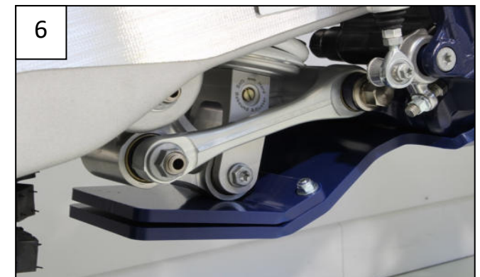
Fix the plastic plate with the Tfhc 6x25mm + M6 Washers + em6f
