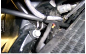
**Brake hose (2):** Reroute the brake hose above the bottom yoke and in front of the stanchion to the brake cylinder. Fix the original fastener to the clutch cable with the attached cable tie.
