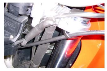
Wiring harness (5&6): Routed as original but not fixed with the original cable ties.
