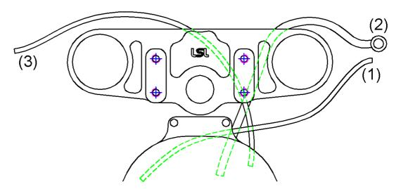
**Throttle cable (1):** To reroute the throttle cable it's necessary to loose the steering damper and the radiator. Route the cable to the right side and guide it behind the right stanchion to the control unit. Use the fastener for the clutch cable, underneath the steering head, to fix the throttle cable and the brake hose. Check throttle cable for free movement on every steering angle.
