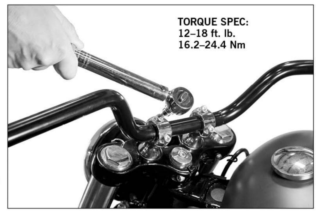
tightening the 1/2" bolts that secure the riser bases to the fork triple tree, check alignment of the handlebar/riser assembly in relation to the motorcycle's front wheel. Move the handlebar/riser assembly back and forth in the triple tree as needed to ensure proper steering alignment. When handlebar alignment is correct, use a torque wrench and 3/4" socket to torque each mounting bolt to 30–40 ft. lb. (40.6–54.2 Nm)
