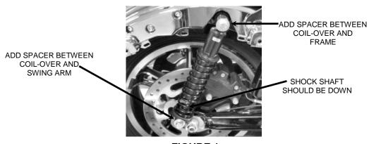
FIGURE 1 **ONLY FOR MODELS EQUIPPED** WITH COIL-OVER SHOCKS
