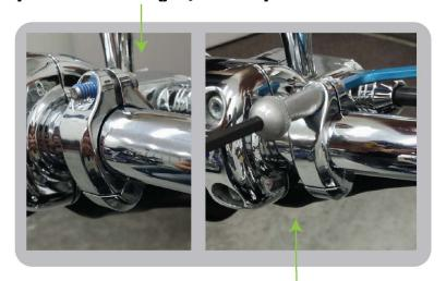
4. Tighten the clamp to the bar using a 3/16" allen in the bolt, and head of the stud. Tighten to 24-26 in-lbs. DO NOT OVER-TIGHTEN!
