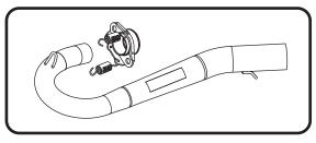
5. Install (No. 1) 22843-105/705, right header into manifold and hook (No. 9) RACE-SPX-1, small exhaust spring onto header using ST-200, spring puller tool supplied in the kit.
