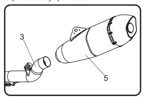
8. Torque tailpipe chassis mount bolt to factory specification and install (No. 8) *RACE-SPS-1*, medium exhaust spring between tailpipe and header as shown on the assembly diagram.
