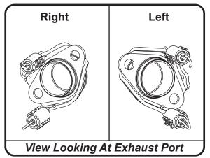
4. Install (No. 1) 22843-104/704, left header into manifold and hook (No. 9) RACE-SPX-1, small exhaust spring onto header using ST-200, spring puller tool supplied in the kit.
