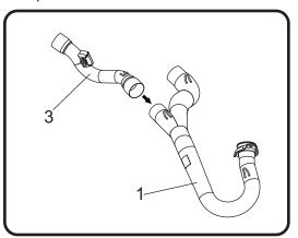
4. Install (No. 5) *right muffler*, over (No. 3) *22583-145/745*, right tailpipe outlet. Align muffler mount bracket to muffler mount and secure using the stock muffler mount bolt and washer. Do not torque at this time.
