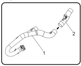
3. Install (No. 3) 22583-145/745, Yoshimura right tailpipe by sliding onto right header outlet. Align tailpipe chassis mount bracket to subframe and secure using the stock chassis mount bolt. Do not torque at this time.
