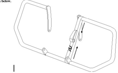
8. Tighten all nuts and bolts. The upper frame mount bolts may be difficult to hold in place while tightening the acorn nuts. This task is made easier by using an air impact wrench to tighten these bolts.
