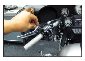
4. Slide on new left side grip until the grip stops against switch housing. Using a transfer punch and a hammer, mark the set screw locations through the threaded holes in the grip.
