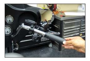
3. Now that the throttle grip is removed verify the throttle sensor fits correctly on handlebar and then slide on new throttle grip on until throttle sensor teeth engage.
