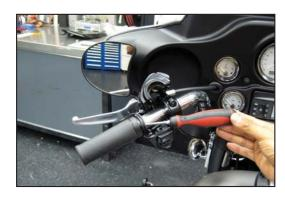
3. Install left side upper and lower switch housing on handle bar. Tighten two T25 TORX screws to factory torque specs.
