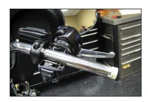
4. Make sure the flange of the throttle grip fits within the throttle/switch housing.
