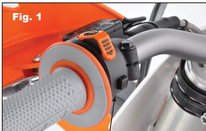
TRAIL TECH IGNITION MAP SWITCH INSTALLED
