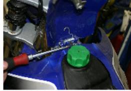
RETIRER LA VIS SUPPORT DU CACHE RÉSERVOIR AVEC UN TOURNEVIS CRUCIFORME.
