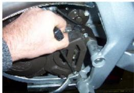
RETIRER AVEC UNE CLÉ A PIPE DE 10 LA VIS DE FIXATION DU SÉLECTEUR ET LE DÉPOSER.
