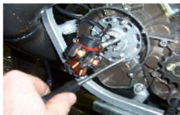
ATTENTION!! LES 3 VIS DE LA PLATINE SONT PARTICULIÈREMENT DIFFICILES À DESSERRER, POUR CE FAIRE, PRÉSENTER UNE CLÉ ALLEN DE 3 ET TAPOTER AVEC UN MARTEAU SUR LA CLÉ AVANT D'ESSAYER DE LA DESSERRER.
