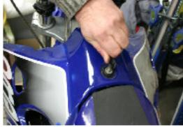
OUVRIRE LE CACHE RÉSERVOIR AVEC LA CLÉ DE CONTACT.
