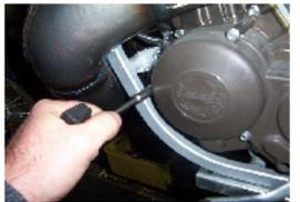
RETIRER LES 3 VIS DE FIXATION DU CARTER D'ALLUMAGE AVEC UNE CLÉ A PIPE DE 8.
