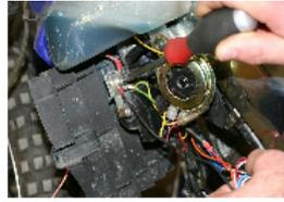
POSITIONNER LA BOBINE HAUTE TENSION A SON EMPLACEMENT D'ORIGINE EN FIXANT A LA MASSE LE CABLE NOIR DU DIAGRAMME ET VERT/JAUNE DU STATOR.
