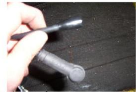
RÉCUPÉRER LE CABLE HAUTE TENSION D'ORIGINE ET PLACER DESSUS LA PROTECTION ANTI HUMIDITÉ FOURNIE AVEC LA BOBINE HAUTE TENSION MVT.
