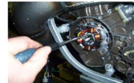
RETIRER LES 3 VIS DE FIXATION DU STATOR AVEC UN TOURNEVIS CRUCIFORME.
