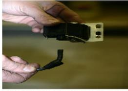
VISSER LE CABLE SUR LA BOBINE HAUTE TENSION ET RABATTRE LA PROTECTION SUR LA BOBINE ET CONNECTER LE CABLE ORANGE DU DIAGRAMME SUR LA COSSE D'ALLIMENTATION DE LA BOBINE.
