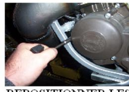
REPOSITIONNER LES 3 VIS DE FIXATION DU CARTER D'ALLUMAGE AVEC UNE CLÉ A PIPE DE 8.
