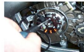
PRÉSENTER LE STATOR MILLÉNIUM SUR SA PLATINE EN PASSANT LA GAINÉ PAR LE TROU DU CARTER ET LE SERRER AVEC LES 3 VIS DE 4 mm FOURNIES AVEC UN TOURNEVIS CRUCIFORME.
