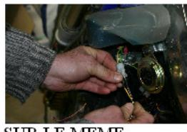
SUR LE MEME CONNECTEUR, BRANCHER LE CABLE NOIR/BLANC DU DIAGRAMME AVEC LE VERT/NOIR DU CONNECTEUR. FIXER LE DIAGRAMME AU DESSUS DE LA BOBINE AVEC UN COLLIER PLASTIQUE ET RASSEMBLER TOUS LES CABLES AVEC 3 COLLIERS PLASTIQUE.
